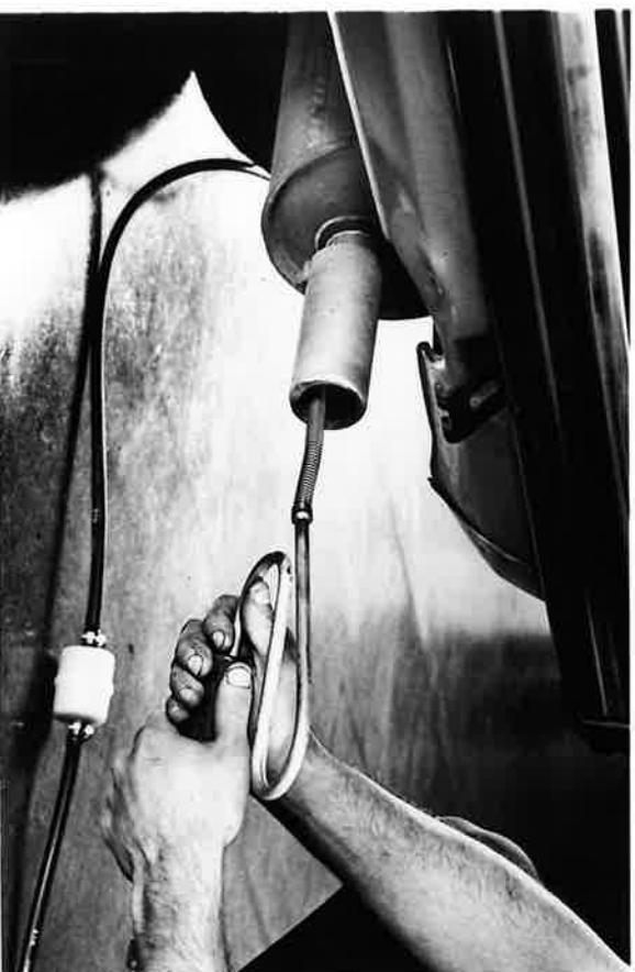
For the new California Smog Check program, a certified mechanic, upper left, makes a thorough visual inspection of the car's emission control system. Then, upper right, he enters data in the tamper-resistant computer analyzer. A probe, lower left, is inserted in the tailpipe to measure emissions. The results, lower right, are printed out and indicate whether the car has passed or failed the inspection.
