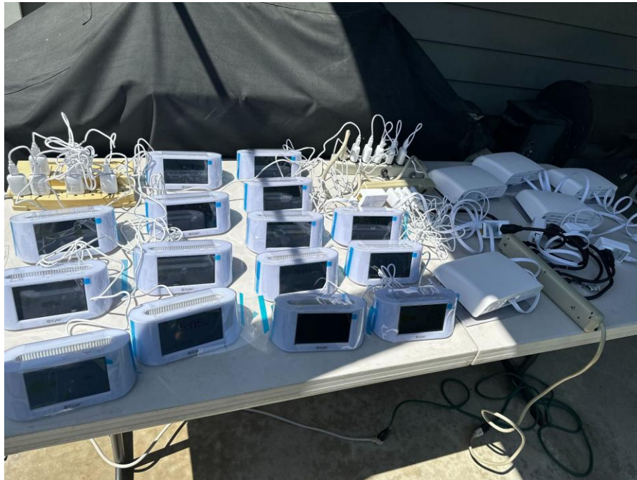
Initial pre-deployment outdoor collocation of all AirVisual Pro and Outdoor devices from June 21 to June 27, 2024.
